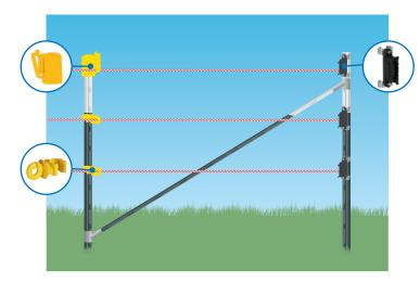
Set includes: 2 x brackets for diagonal strut, incl. fastening screws and protective caps
