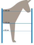
Electric Fence for Jumping Horses Recommendation: Rope, Wide Tape up to 40 mm
