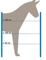
Electric Fence for Big Horses Recommendation: rope or tape up to 40 mm
